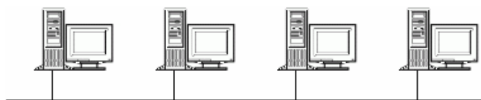
Figure 1.4: The Bus Topology
